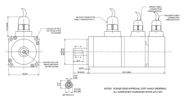
200 Watts Motors with brake
